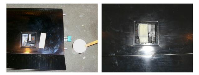
To remove, Dremel the bridge free and remove it, and then pop the servo free of the upper skin by twisting it.
