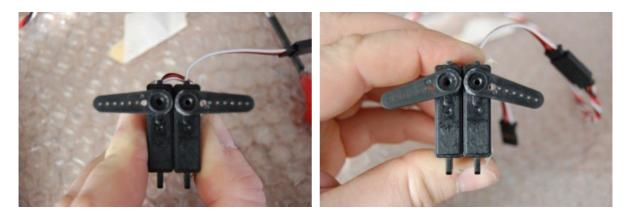
Once you have the holes in the arms, centre up your servos as shown. Ideally, do this with a servo tester. Note the subtrim numbers for each servo. Doing it with the arms untrimmed and left long makes it easy to get them symmetrically placed by eye.
