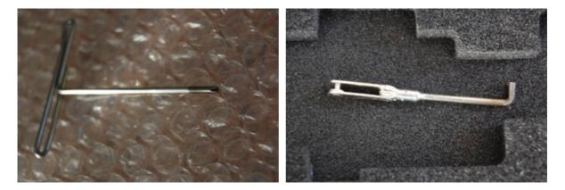
To thread it into the servo arm, drill a 1.6mm hole 6mm from the centre of the hub.
