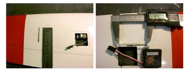
Cut the supplied pushrod to the length shown. Heat it up with a lighter or similar in a vice and slowly bend the threaded end as shown so that the length of the portion which goes through the servo arm is 7mm including the thickness of the pushrod. This is so that it will clear the servo casing when the servo is at full rotation.
