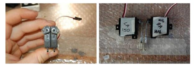
Then trim the servo arms as shown and install the linkages as shown above.
