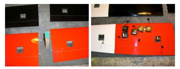
CA a piece of 80 grit sandpaper to a block as shown as use it to sand the inside of the servo bays lightly to prepare them for glue.
