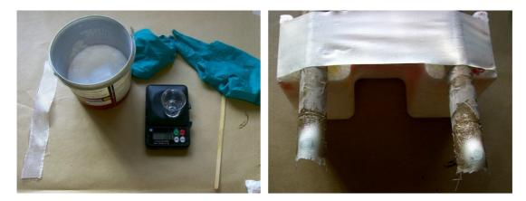
Mix up some epoxy and thickener and splooge around the nut from the underside. Cap it off with a layer of 100g glass cloth if you have some as shown. When dry, the bolt will easily unscrew due to the grease/ wax you put on the threads. That's your tube prepared! Now let's prepare the fuselage for the ballast tube.
