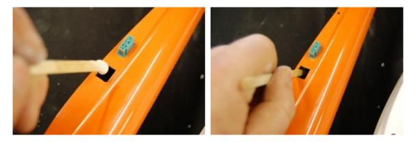
Securing the wing-side can be done as an automating connection, but the simplest way to do it is to simply leave the wing side loose and plug it on manually when sliding the wing on.
