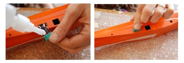
Then, through the wing joiner hole, put some thickened epoxy onto the back of the connectors to secure them really well.
