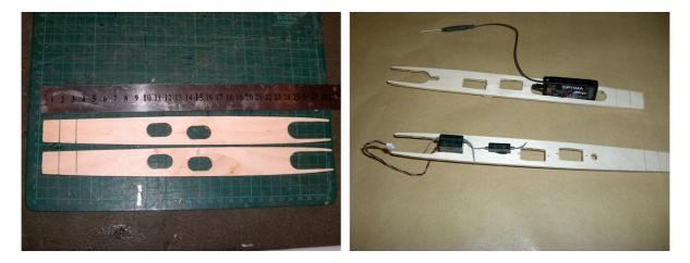
Note the marks at the rear of the tray. They show the position of the wing joiner. The tray runs underneath the wing joiner with enough clearance for the snakes to also go under the joiner. It is wise to put your fuselage wiring loom in place prior to gluing the tray in as this saves having to try to thread it through after the tray is in position!
