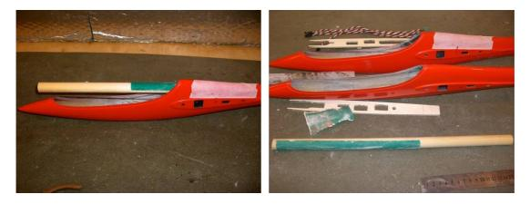
Glue some 80 grit sand paper to some 19mm dowel. If you don't have any dowel to hand, then you can just wrap some 80 grit paper around the actual ballast tube and secure it at one end with a wrap of masking tape. Use this to lightly sand the inside of the fuselage for the length of the ballast tube. Also, use some loose 80 grit sand paper to prepare the inside of the canopy area for gluing in the servo tray.
