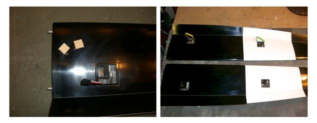
Then install the servo to the wing as shown. Ensure that the wiring loom is loose installed to the servos prior to gluing. Route the loom in FRONT of the servos to ensure that it does not interfere with the linkage. Put some heatshrink over the connectors to ensure that they remain secure. Bring the green mpx connector out through the hole provided in the wing root.
