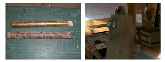
First, cut the tube to 195mm long from the inside of the rear stopper. Shape the front as shown. This fits  $5 \times 35$ mm long slugs plus a 20mm retainer.
